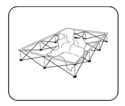
Attach the rest of the graphic by working your way around the frame. Make sure graphic is pulled taut while attaching the velcro.
