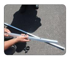
**Step 10**Grab 2 of the larger poles and 1 small pole and connect them together creating 1 rail that slides through the pole pocket on the bottom of the Backwall graphic.
